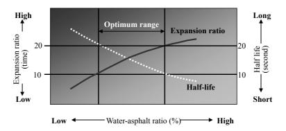
Figure 1: Relationship between water-asphalt ratio and foaming properties
