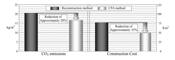
Figure 10: Comparison chart of carbon-dioxide emissions & construction cost
