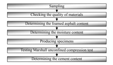
Figure 4: Flowchart of CFA mix design
