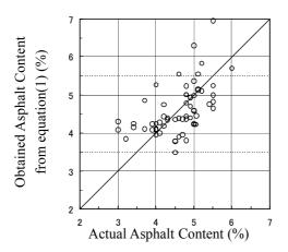
Figure 5: Relationship between actual asphalt content and obtained one from equation (1)
