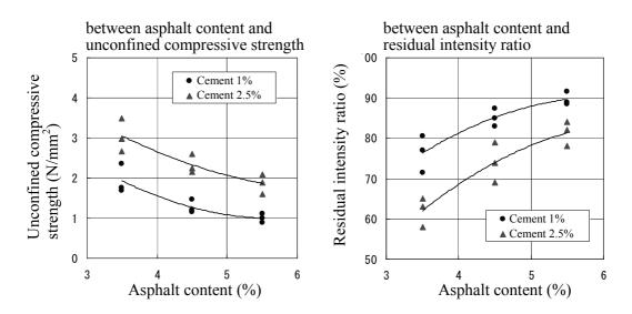
Figure 7: Relationship between asphalt content and properties
