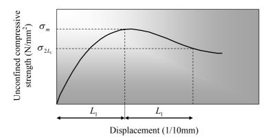
Figure 6: Relationship curve of displacement and unconfined compressive strength
